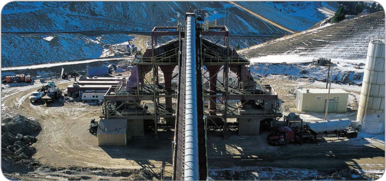
Primary transportation of gold bearing ore from the crusher to the heap leach pads
